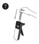
Insert the whole body of the LuciPac into the measurement chamber of the Lumitester.
