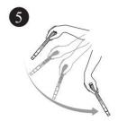
Shake the whole body of the LuciPac a few times so that the liquid in the capsule falls into the test tube (C)
