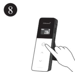
8 Press the "START" key. Results are obtained in 10 seconds.
